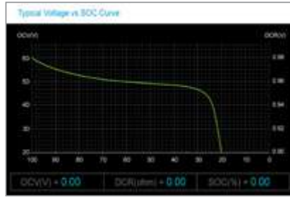
Battery characteristics V-SOC curve setting screen
