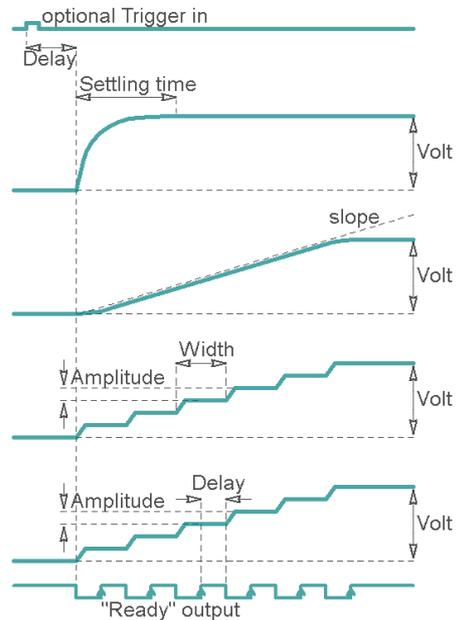
Whatever the chosen mode, a “Ready” output signal allows to optimize settling synchronization. “Ready” comparator tracks the gap between the expected voltage and the actual sensed voltage:
