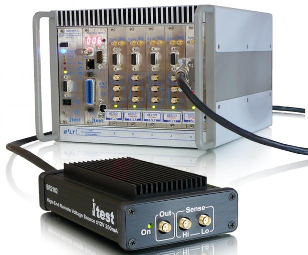
Example of a BE103 5-slot BILT chassis fitted with 4 BE2101 (front panel output) and one BE2102 (remote source)
