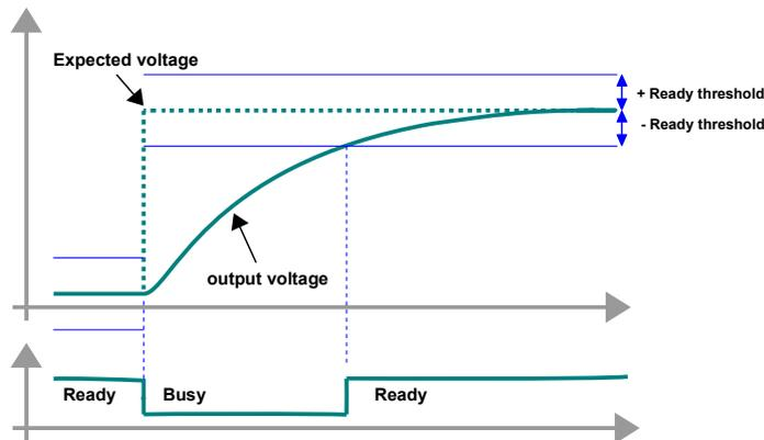
Following the actuation of a new voltage setting, it allows to trigger any measurement process as soon as the output settles within a requested amplitude.
