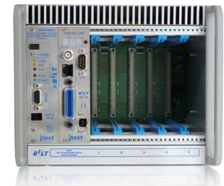
Empty 5-slot BE103 BILT chassis
