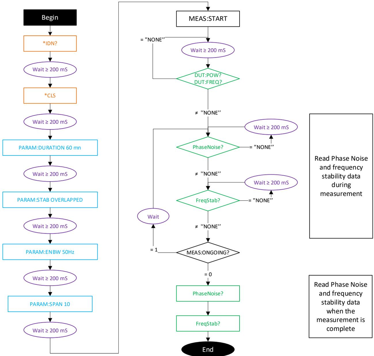
Figure 3 : Remote control example 2
