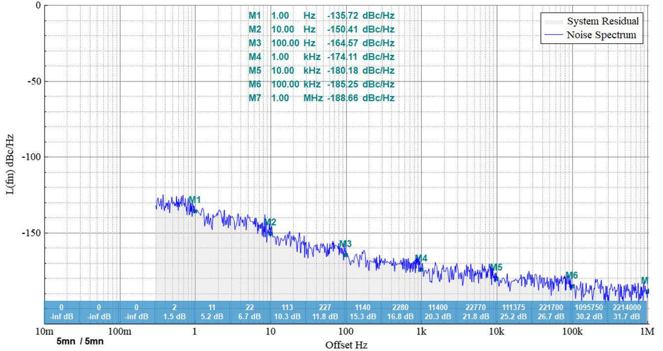
Typical 10 MHz residual Phase Noise, 5min measurement time
