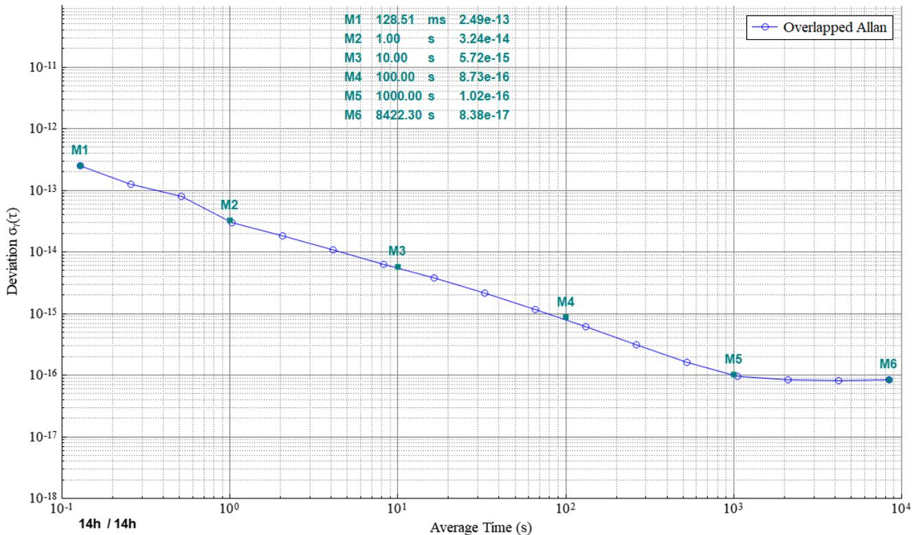
10 MHz / 14H measurement time Residual Overlapped Allan Deviation ENBW=5Hz
