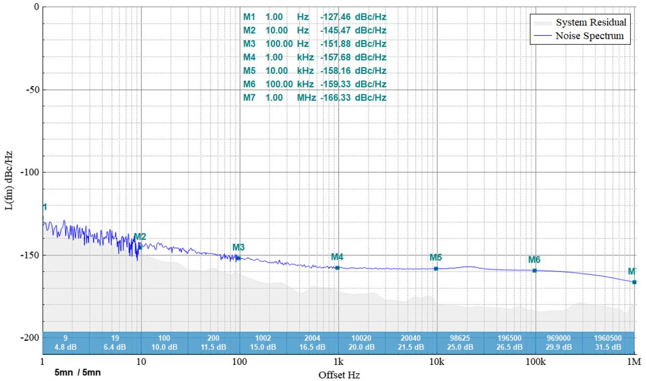
5 MHz OCXO / 5 min measurement time phase noise plot
