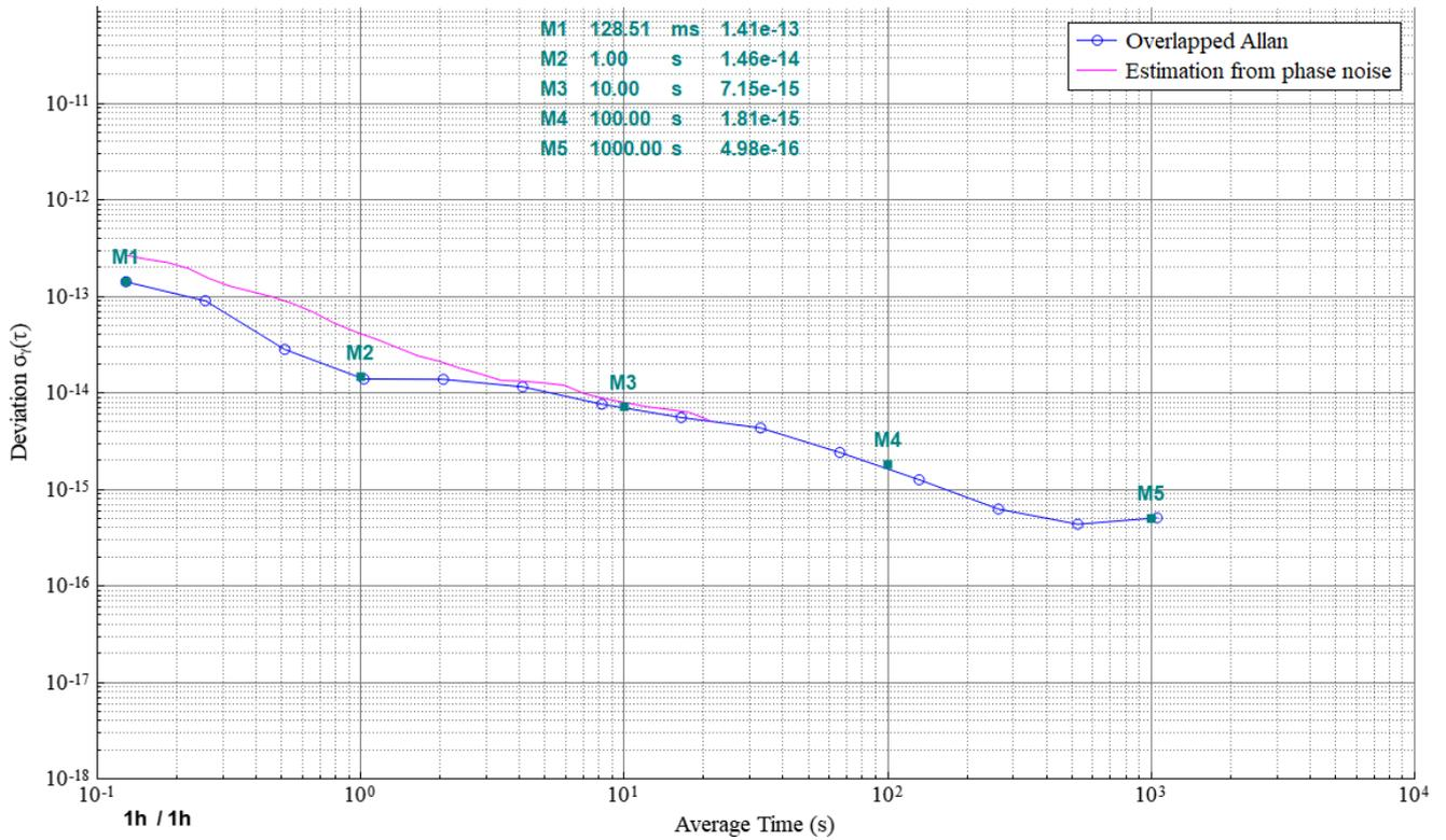
5 MHz / 60min measurement time Residual Overlapped Allan cross variance Deviation ENBW=5Hz
