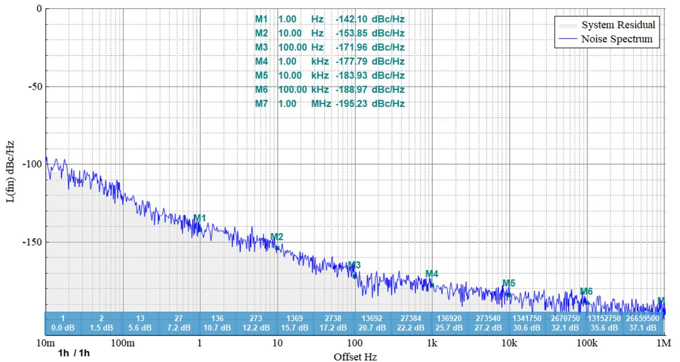
Typical 10 MHz residual Phase Noise, 60 min measurement time
