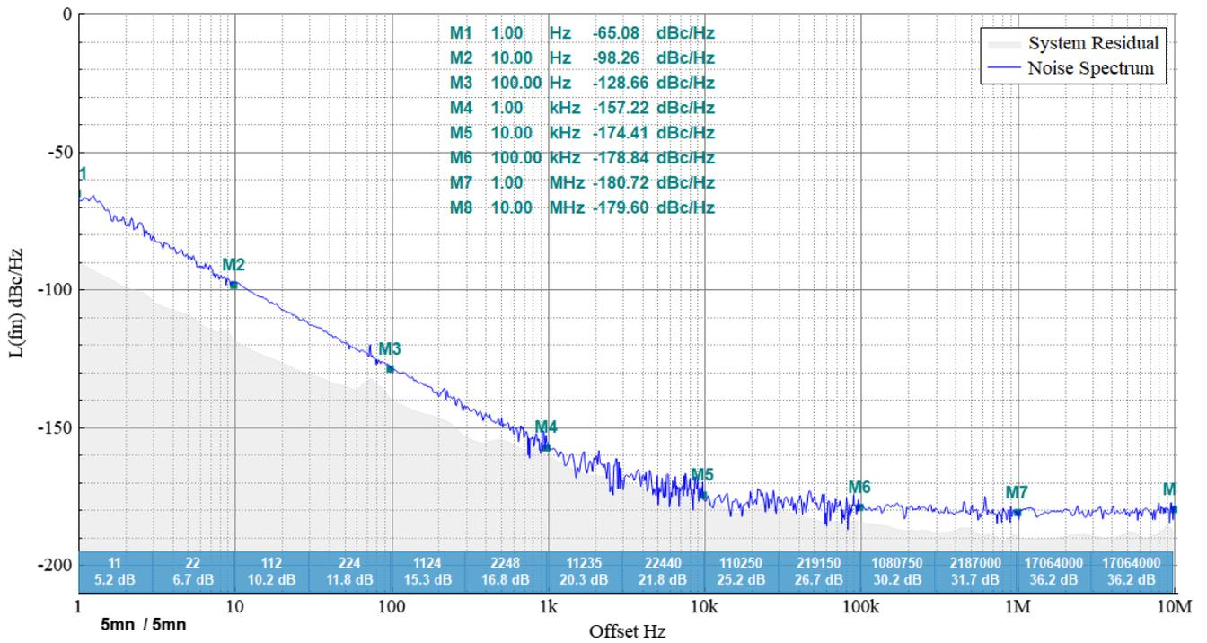
100 MHz OCXO / 5 min measurement time phase noise plot
