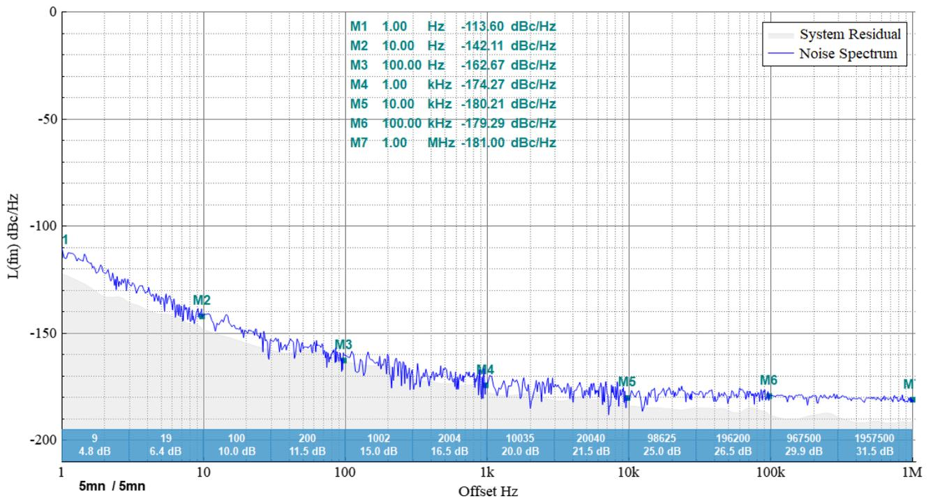
10 MHz OCXO / 5 min measurement time phase noise plot
