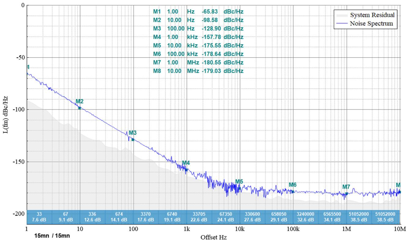
100 MHz OCXO / 15 min measurement time phase noise plot
