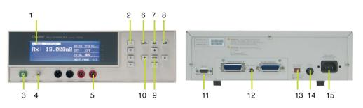
1.LCD Display 2. Function Keys 3. Power Switch 4. Ground Terminal 5. Unknown Test Terminal 6.MEAS DISPLAY Key 7.MAIN INDEX Key 8.SYSTEM SETUP Key 9. TRIGGER Key 10.Cursor Keys 11.RS232 Interface 12. GPIB and Handler Interface with Temperature Compensation (A165013ption) 13. Line Voltage Selector 14. Fuse 15. AC Line Input
