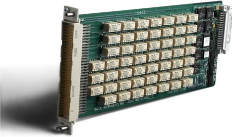
The Racal Instruments™ 1260-117/117A is a 52/20-channel, SPDT (Form C) plug-in switch card for the Adapt-a-Switch™ platform. It quickly and easily plugs into the front of Racal Instruments™ 1260-100 and 1260-101 VXI Adapt-a-Switch™ carriers or the Racal Instruments™ 1256 GPIB/Ethernet and 1256L (LXI Core 2011 Compliant) switching mainframes.
