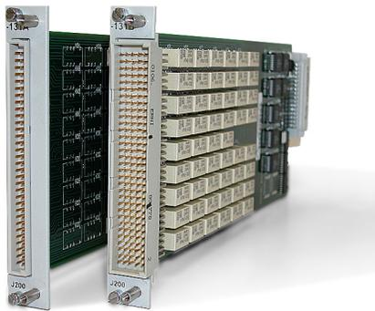
The Racal Instruments™ 1260-131A/B is a general-purpose, SP4T binary tree with a 200 MHz bandwidth (-3 dB). The 1-A “A” version is for lower density/cost.
