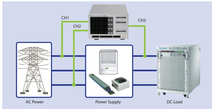
With the wiring mode set as 1P2W, the 66204 Power Meter has the capability of performing up to 4 simultaneous power measurements as shown. The meters are also designed to comply with power measurement requirements in accordance to many international standards such as Energy Star/EN 50564/IEC 62301/ErP.
