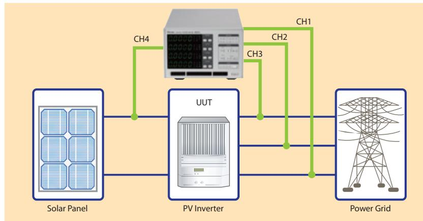
User could implement 3P3W (Three Phase Three Wire) wiring mode for three phase power measurement application. Such as Power Supplies.
