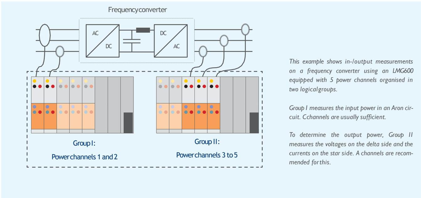
This example shows in-/output measurements on a frequency converter using an LMG600 equipped with 5 power channels organised in two logical groups.
