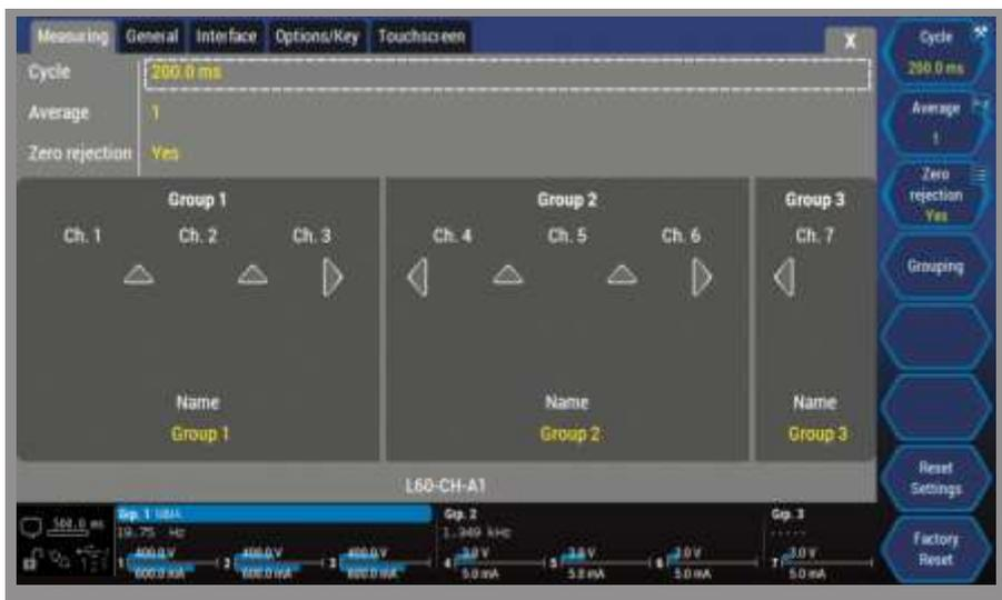
This screenshot depicts an example for logical grouping of an LMG600 fitted with 7 power channels, e.g. for measuring an electric drive. Group 1 & 2, with three channels each, could comprise the 3-phase input/output connections, while the single-channel Group 3 might represent the DLink.
