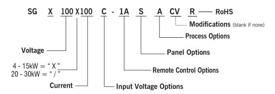
(For units with greater than 3 digits, Voltage/Current is represented in numeric format, e.g., above "100" represents 100A. For units at 1000 and above, the voltage is represented by the format "XKX", e.g, 1K2 = 1200V and 1K0 = 1000V)
