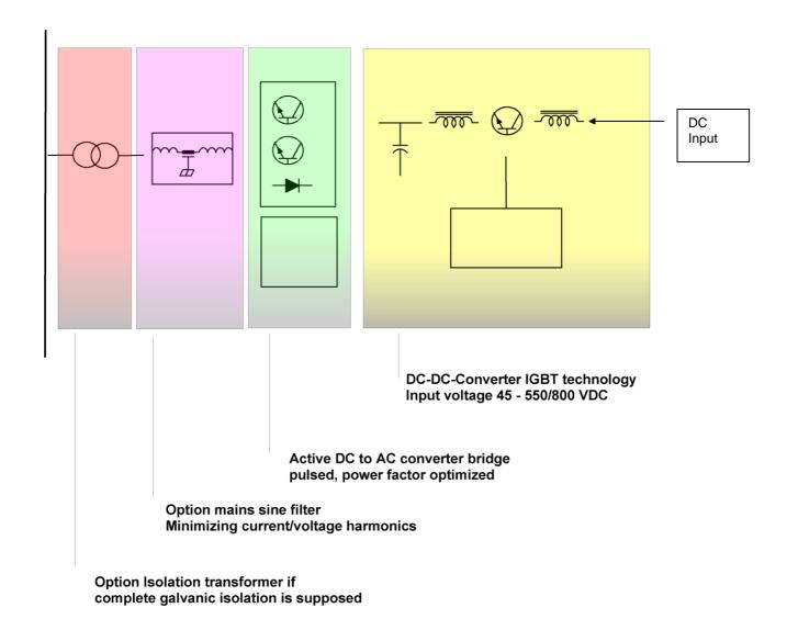
The system power rating is calculated at the desired DC input voltage. The corresponding DC input current can be drawn from max. DC down to less than 45 V DC.
