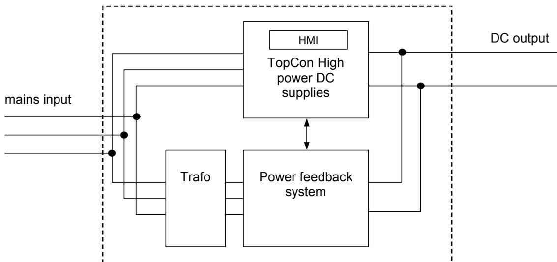
**Basic system diagram of REGATRON ReGen system**
