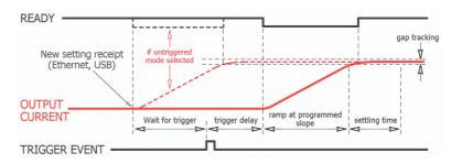
In any case, the current setting update is processed according to a programmable slope, useful for maintaining linear operation with large steps and large inductors.
