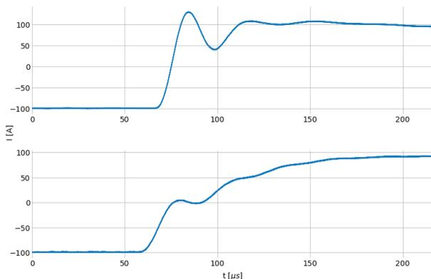
Figure 2: Parameterization example: set-value step currents. -97...97 A@333VDC in <50 µs with overshoot (top), in <200 µs w/o overshoot (bottom).
